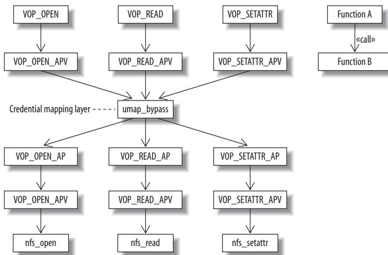
FIGURE 17-3. Routing system calls through a bypass function
