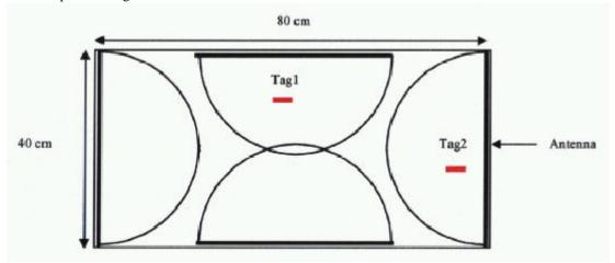
Figure 5: Shopping cart top coverage with four readers
