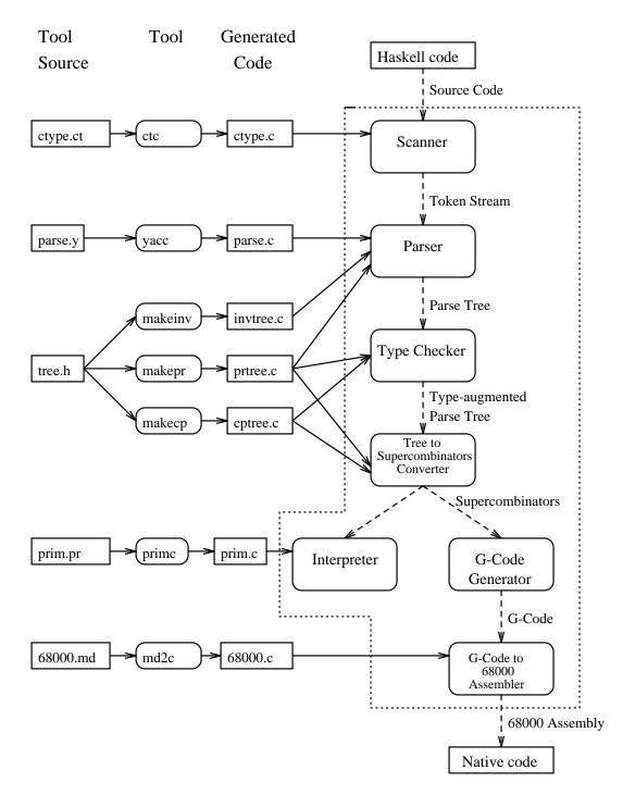
Figure 1: System Construction, Structure and Cooperation of the Components
