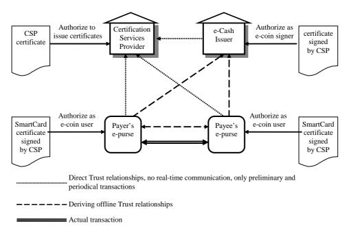
Fig. 2. Off-line Trust Model
