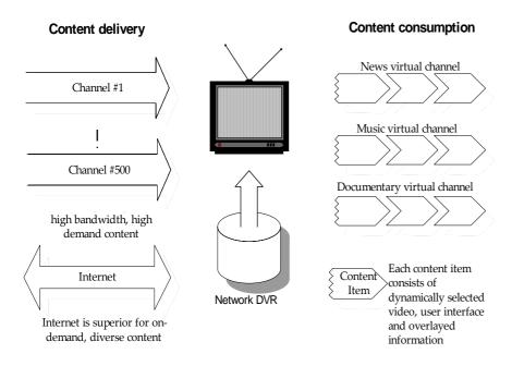
Figure 1 The network DVR as a virtual channel provider
