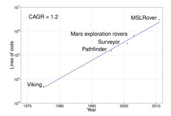
Figure 1. Software growth over the series of NASA Mars missions.
